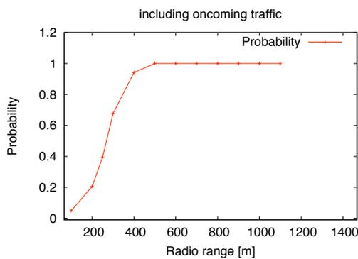
Figure 4: Probability of two nodes to be able to communicate w.r.t. radio range
